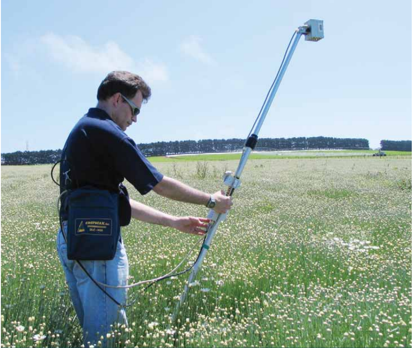
Dr Frank Hay assesses Phoma disease at a fungicide trial in pyrethrum at Kindred, TAS, with a multispectral radiometer. The radiometer measures net reflectance from the crop canopy at different wavelengths. Some wavelengths are well correlated with green leaf area and conversely the amount of damage due to disease. It is used as a rapid means of assessing disease in plots as a back up to visual assessments.
