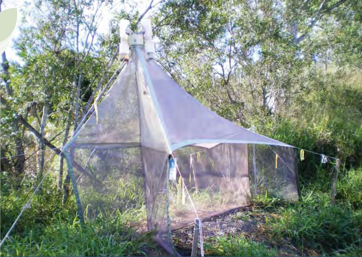
Malaise traps are placed across insect flight paths to intercept and collect insects. The traps indicate from which direction insects have come, and this data is used to ascertain whether pests are moving from vegetation into crops or vice versa. Images supplied by CSIRO.
