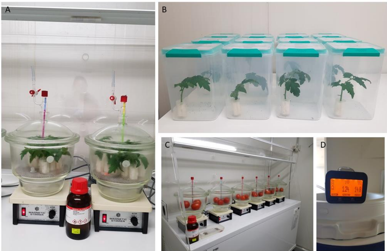
EF fumigation trials in desiccators (A), tomato leaves with TPP life-stages (B), fumigation on fruit (C), and portable gas detector Microtector II G-460 for EF and CO 2 (D).
