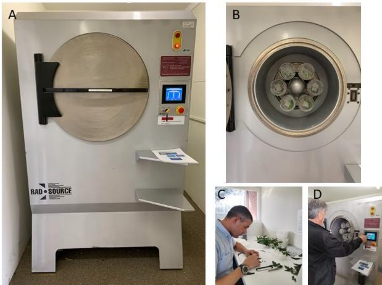
Radsource RS2400Q X-ray irradiator (A) loaded with TPP samples (B), staff preparing TPP samples (C) and operating the irradiator (D).
