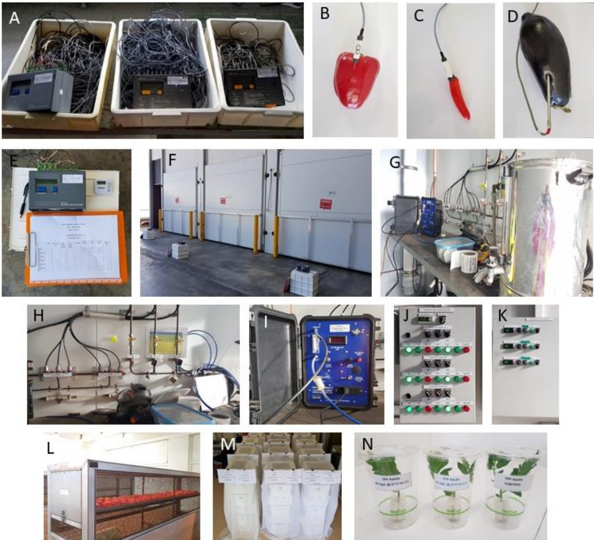
Temperature probes prepared for fumigation trials (A), probes inserted into fruit (B, C, D), temperature data being recorded during trials (E), trials in progress inside fumigation rooms (F), vapouriser and gas line setup (G), gas lines for each room (H), Fumiscoper (I), ventilation (J) and temperature (K) control systems, natural infestation of capsicum (L), setup of capsicum infested with Medfly eggs in controlled environment (M) and TPP cup cage assemblies prepared for fumigation trials.
