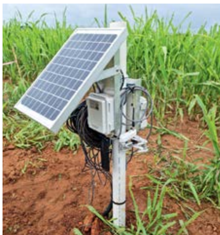
Soil moisture sensors with communications node. Right. Control Tower in use at AustChilli. Image Applied Horticultural Research, 2022.
