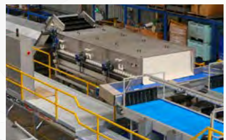
edp stainless steel flat-bed washing unit 1800mm wide x 38 row nylon brushes
