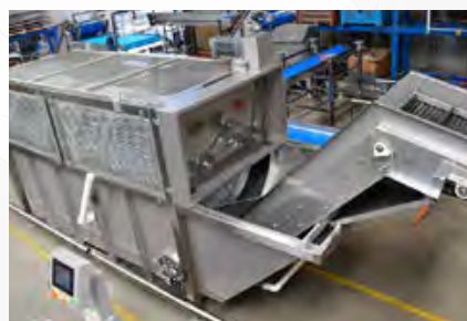
edp stainless steel barrel washer 1200mm dia. x 3600 long
