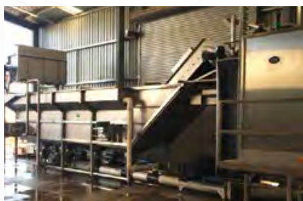
edp 5 tonne wet hopper featuring programmable auto flashing vales
