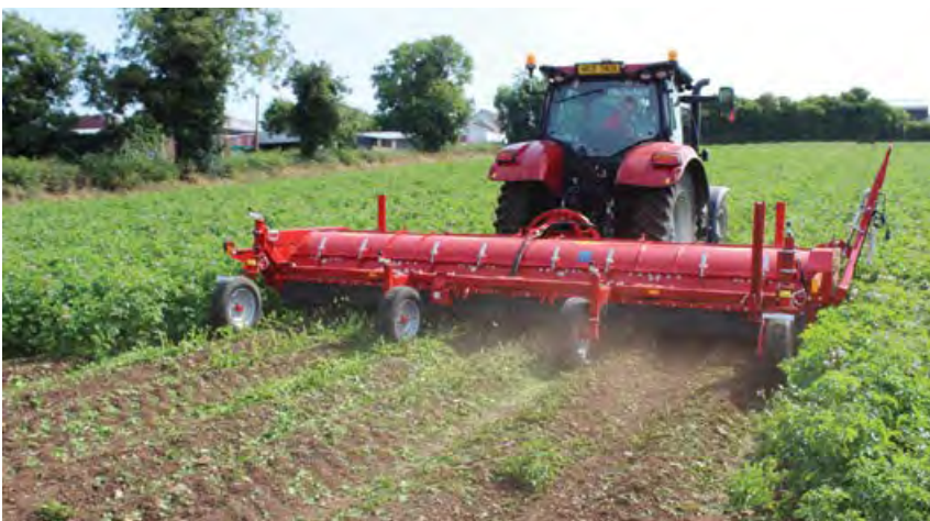
Figure 5. This Grimme mechanical topper crushes and chops the plant haulm and deposits the trash in the interrow, leaving the plant stems exposed for further treatment. Image: R Halleron, Agriland.
