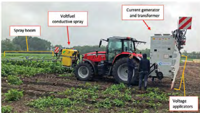
Figure 4. The CROP.ZONE system for vine termination combines an electrically conductive spray with voltage applicators, electrocuting the potato plants. This collapses the plant vascular system, starving the leaves of water and nutrients.
