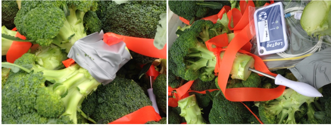
Figure 19 Broccoli with i-button Thermochron (L) or Logtag probe inserted into the stem.
