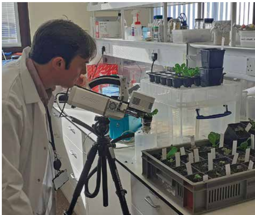
Dr Rob Hancock at work in the lab, measuring photosynthesis using infrared gas exchange.
