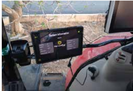
Instead of a load cell, the HarvestEye system uses a camera mounted over the belt, plus control panel in the tractor cab.
