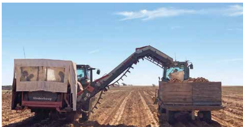
Potato weight is usually recorded using a load cell on the harvesting belt. This is combined with GPS tracking data and conveyor speed to calculate total yield and generate a yield map.
